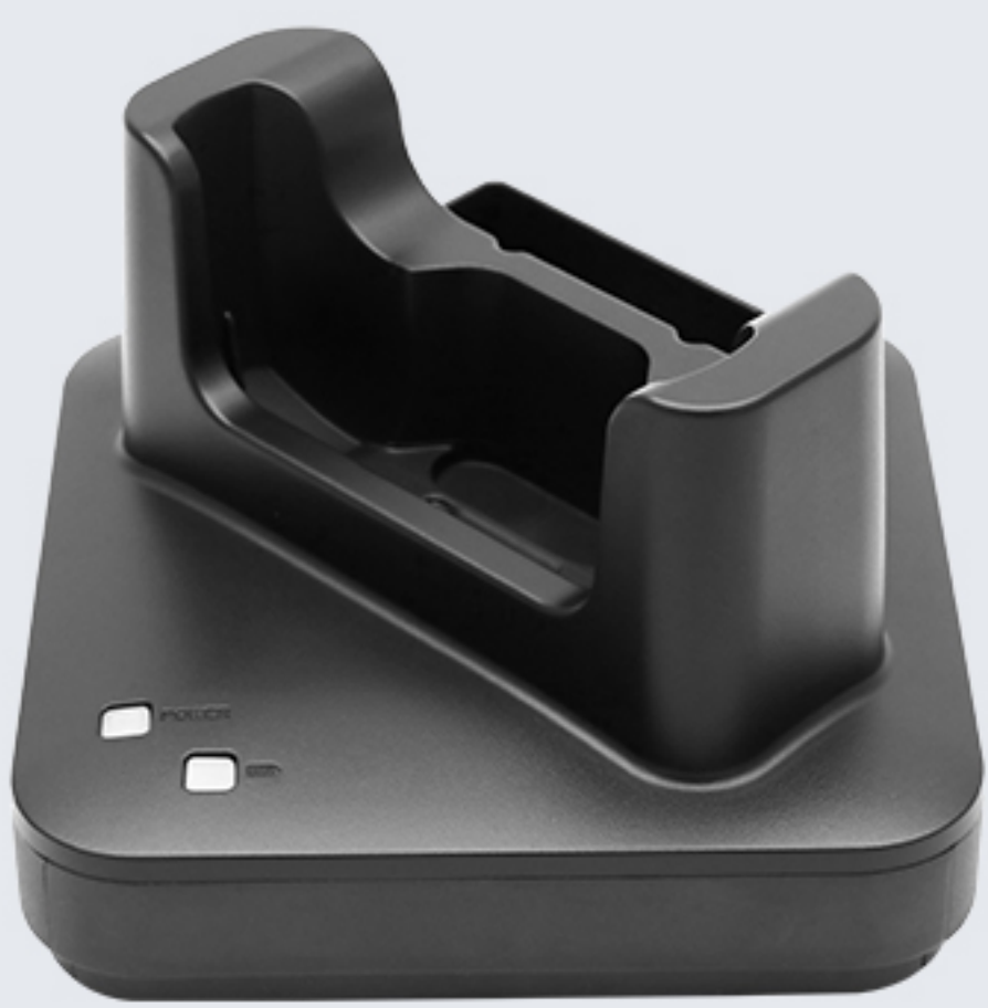
CRD-C95-RBC Charging cradle for device, w/DC use with 12V2A adapter.
